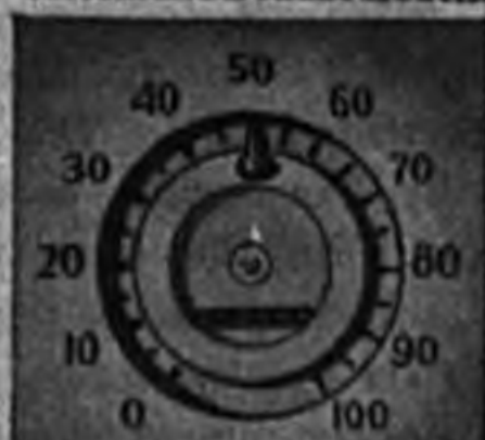
Up to 30 miles an hour the light on the Speedometer Needle shows green . . . 30 to 50 m.p.h., amber . . . and from 50 m.p.h., a warning red.
