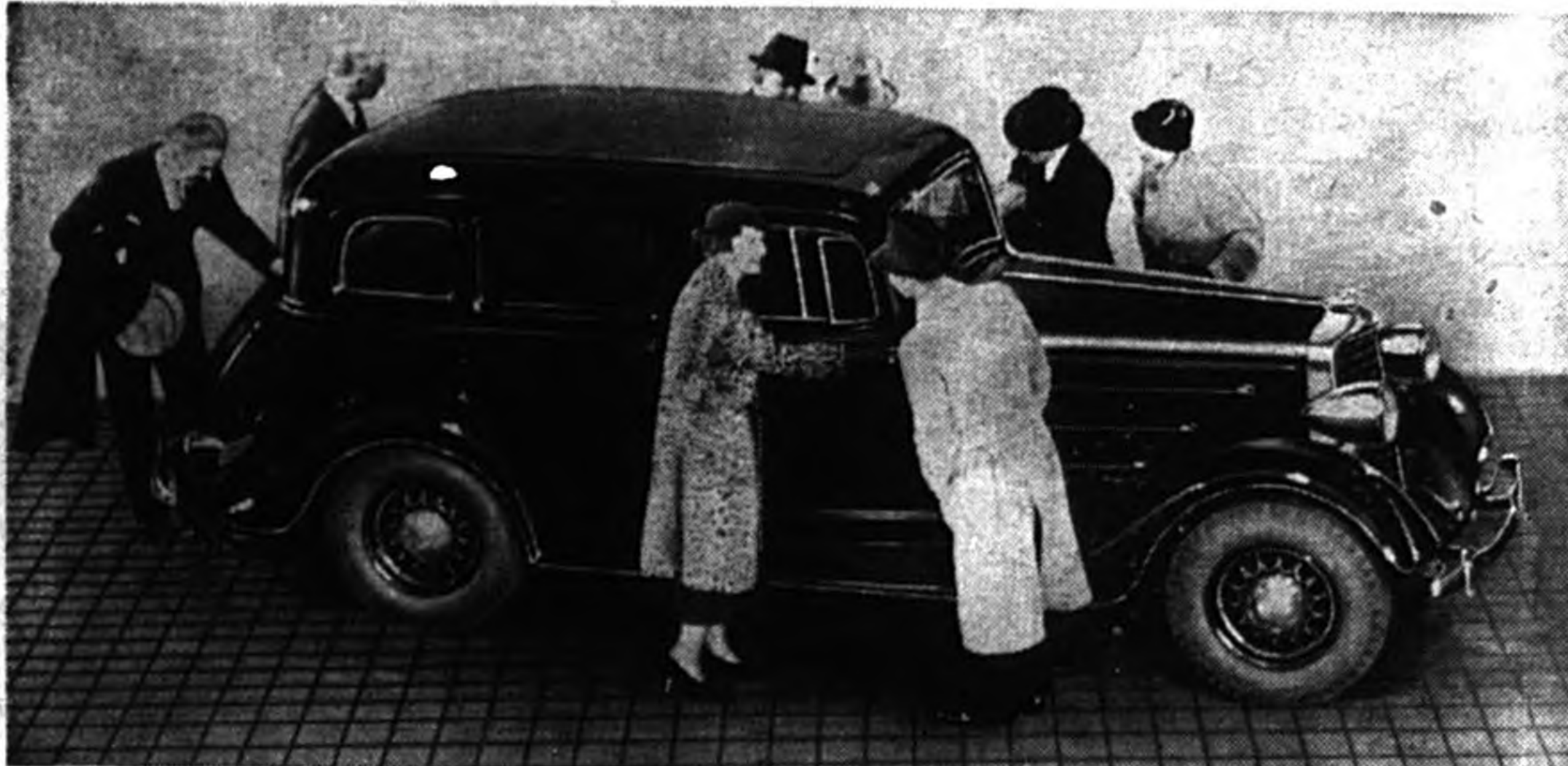
New 1934 117" wheelbase Dodge Six . . . bigger, stronger, more rugged than ever . . . with independent front springs, Floating Power, all-steel body, 7-Point Ventilation, built in luggage compartment.
